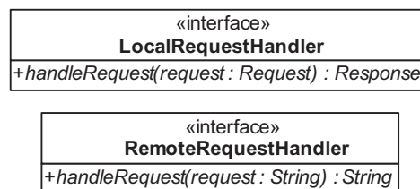
Figure 2.3: Handlers implement the service specific requirements for communication with a remote system.
